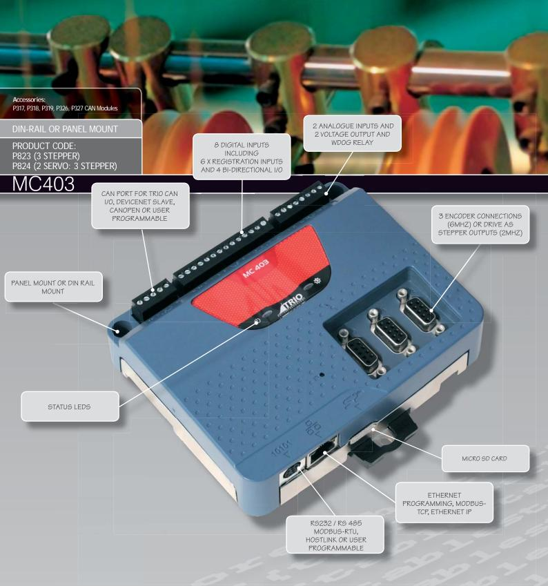
The MC403 is a high specification *Motion Coordinator* using a high performance ARM11 processor and provides up to 2 axes of servo plus a master encoder axis or up to 3 axes of stepper control. All 3 encoder ports can be either incremental or one of three popular absolute encoder types; SSI, Tamagawa or Endat, additionally the 3rd axis can be used as a stepper, reference encoder input or a sync encoder output.
