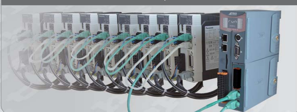
MC464 can control up to 64 Axes
