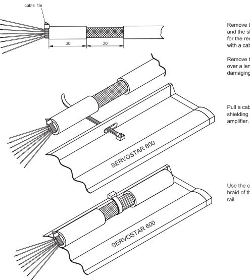
Remove the outer covering of the cable and the shielding braid from the cores for the required length. Secure the cores with a cable tie.
