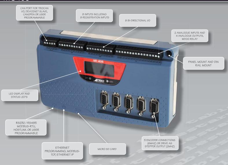
The MC405 is a high specification Motion Coordinator using a high performance ARM11 processor and provides up to 4 axes of servo plus a master encoder axis or up to 5 axes of stepper control. All 5 encoder ports can be either incremental or one of three popular absolute encoder types; SSI, Tamagawa or Endat, additionally the 5th axis can be used as a stepper, reference encoder input or a sync encoder output.
