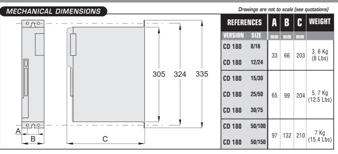
All dimensions are in mm To obtain the dimensions in INCHES, divide mm by 25.4 E
