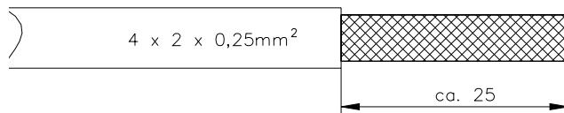
Strip off about 25mm of the outer insulation, taking care not to damage the shielding braid.
